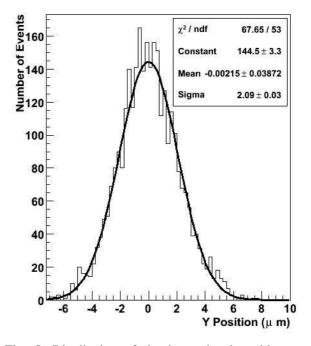
Fig. 5: Distribution of the laser signal positions as determined from 4000 events taken within 40 seconds.
