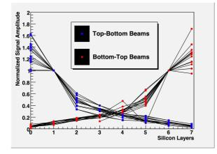
Fig. 7: Normalized laser signal amplitude as a function of silicon tracker layer number where top-bottom (bottom-top) beams are indicated by blue (red) dots.
