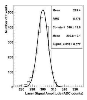
Fig. 3: Typical laser signal amplitude distribution sampled over 4000 events of one of the 40 laser rays of the AMS-2 silicon tracker laser alignment system.
