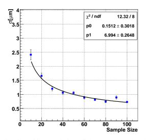
Fig. 6: Position resolution of the AMS-2 tracker laser alignment system as a function of the number of laser signal events used for the analysis.
