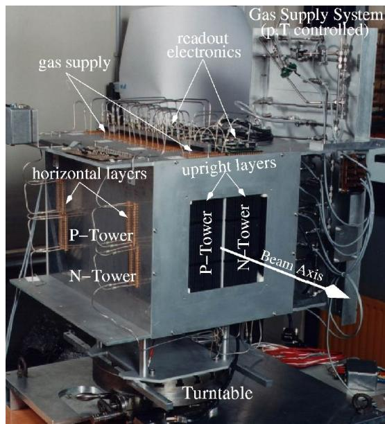
TRD prototype prepared for testbeam (2000)
