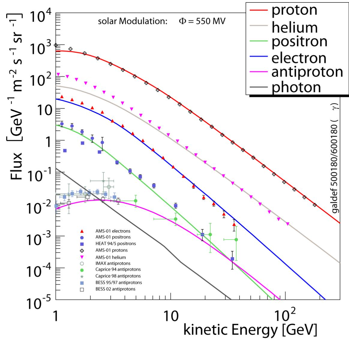
e.g. at 40 GeV:  $10^{-4}\text{GeV}^{-1}\text{m}^{-2}\text{sr}^{-1}\text{s}^{-1} \times (100 \times 24 \times 3600)\text{s} \times 0.4 \text{ m}^2\text{sr} = 344 \text{ e}^+/\text{GeV}$
