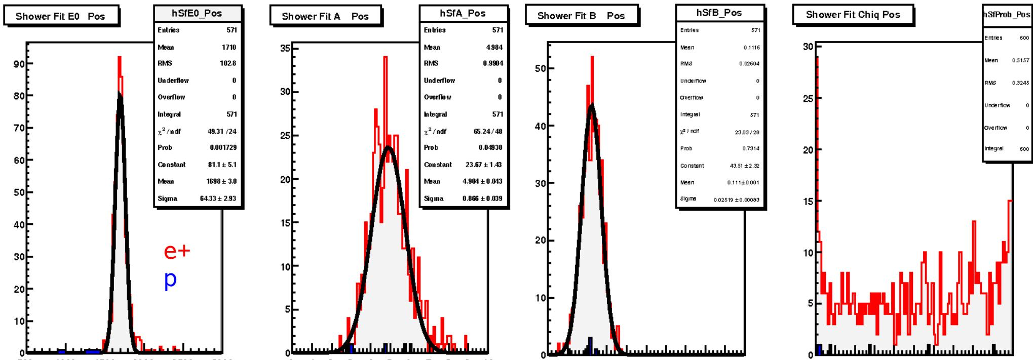
shower shape fits for parameters  $E_0$ ,  $a$ ,  $b$  from fast simulation
