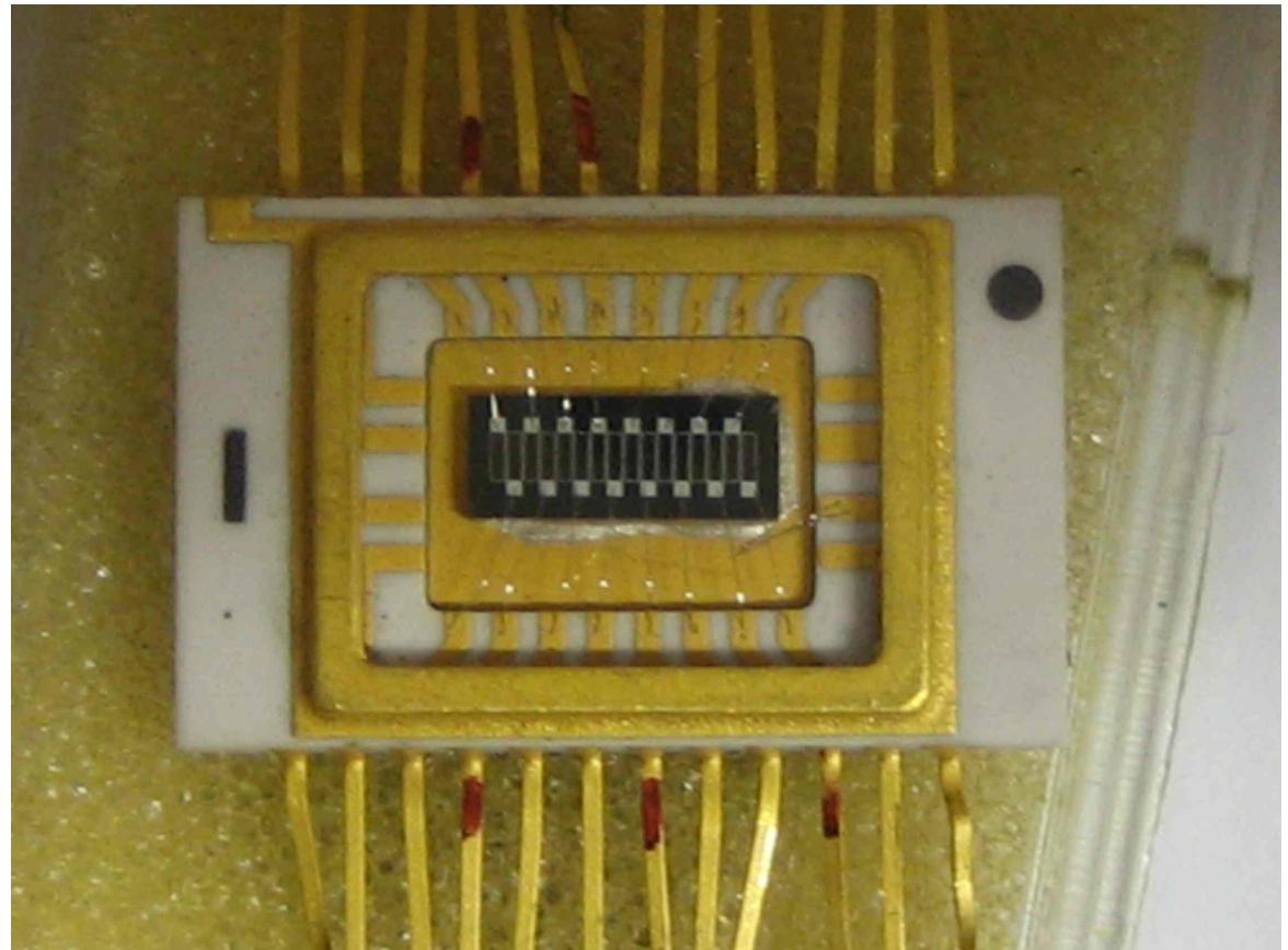
16x1 silicon photomultiplier, strip width 380 µm
