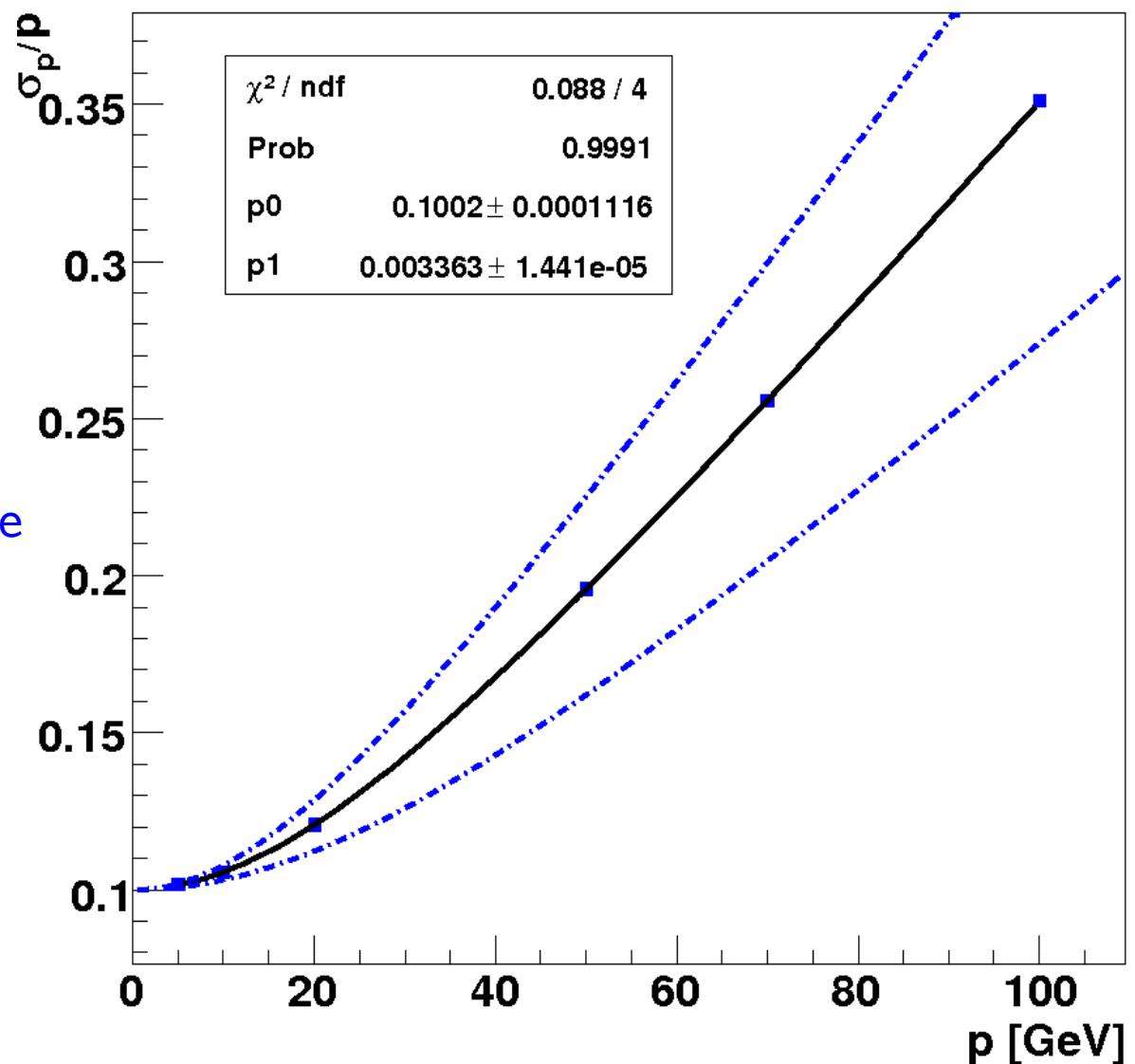
momentum resolution for 4x1 readout and stereo angle from fast simulation
