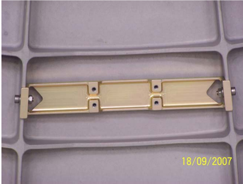
Photo 3: 4 Special Connector Supports (drawing number: ams02-08-3007, ams02-08-3008, ams02-08-3009, ams02-08-3010, ams02-08-3014 and ams02-08-3015) for sectors 5, 11, 21 and 27 on Z- side
