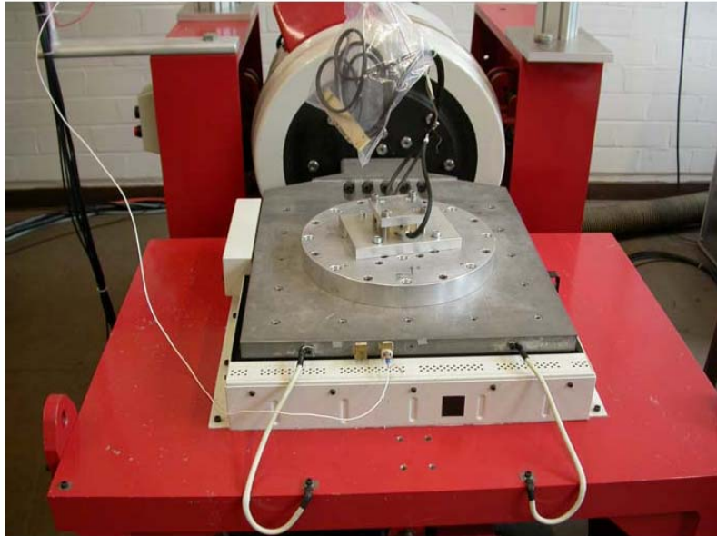
Fig. 1 Thermostat Box 02 mounted on Vibration-table in x-axis
