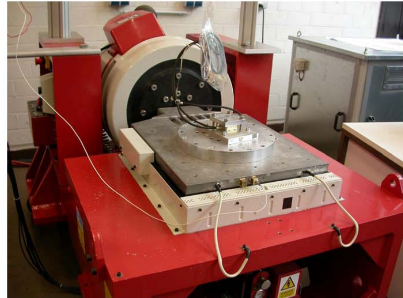
Fig. 4 ThermoStat Box 02 mounted on Vibration-table in y-axis
