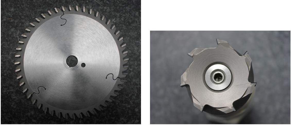
Figure 3.19: Tools: Saw blade for pre-cut (left) and a diamond head for final optical cut (right).
