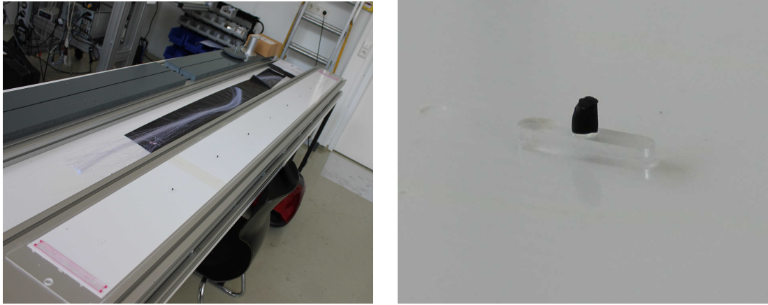
Figure 3.16: Optimization of casting process parameters: Casted dummy with EPOTEK 301, zoomed view of one alignment pin.
