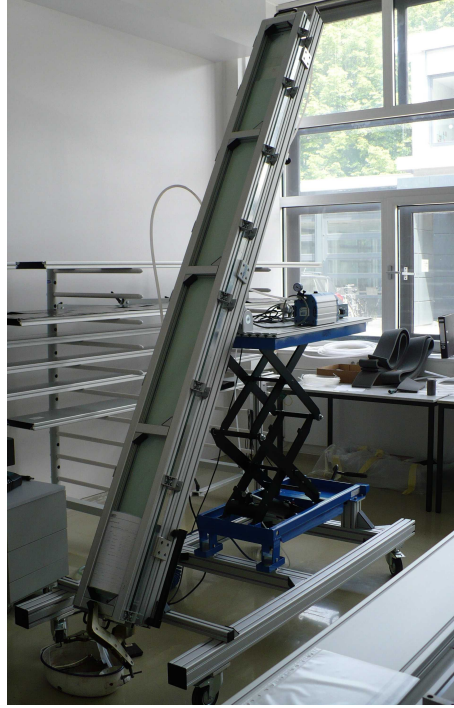
Figure 3.14: Step 9: Filling of glue into casting jig
