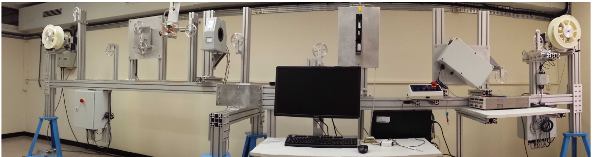
Figure 2.7: Panoramic photo of the FDS at CERN. The total width of the set-up is 6 m.
