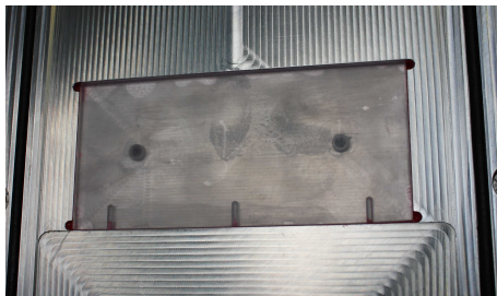
Figure 3.13: Step 5: Placing of endpiece on readout side (left) and mirror side (right) in casting mold and sealed with Latex
