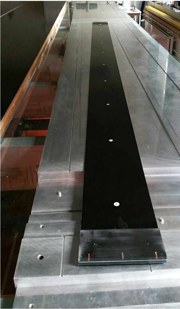
Fig. 3. A six-layer scintillating fibre mat laminated with a black Kapton XC foil and with endpieces glued to it. The SiPM arrays and the mirrors are mounted to the endpieces.
