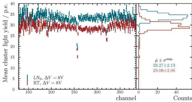
Fig. 7. Light yield measurement of a 6 layer fibre mat with SiPM arrays placed in a vacuum box before and after cool down to cryogenic temperatures.
