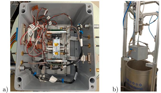
Fig. 3. (a) ToF-prototype positioned in light- and air-tight box. (b) Box inside the liquid nitrogen bath.
