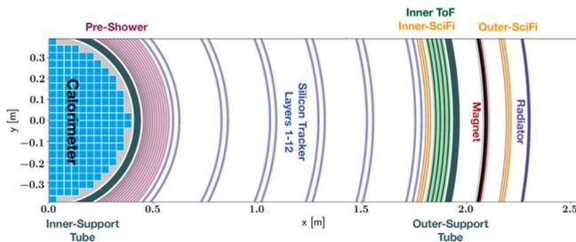
Fig. 2. Cross section of the AMS-100 detector with its cylindrical sub-detector layers.
