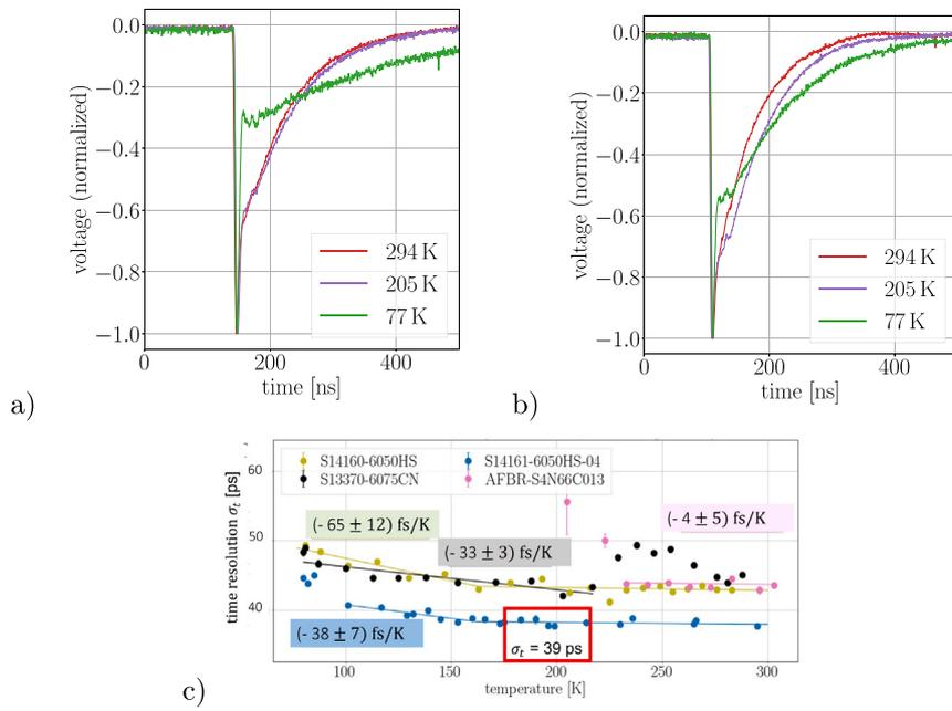
Fig. 4. (a) Signal shape at different temperatures for SiPMs with poly-silicon quench resistors, (b) Signal shape at different temperatures for SiPMs with metal quench resistors. (c) Temperature dependence of the time resolution  $\sigma_t$  for all tested SiPMs. The red box indicates the operational temperature range.
