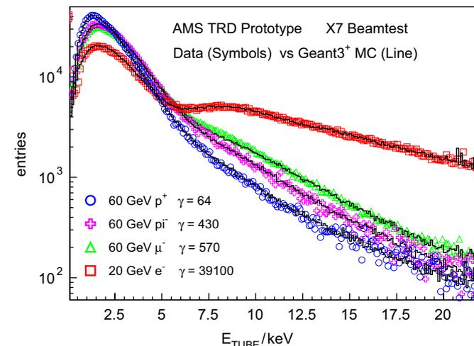
Fig. 7. AMS-02 TRD straw tube energy spectra for clean single tracks.
