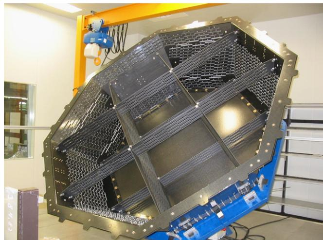
Fig. 3. AMS-02 TRD octagon support structure.
