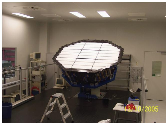
Fig. 4. AMS-02 TRD octagon structure with all 328 straw modules integrated.
