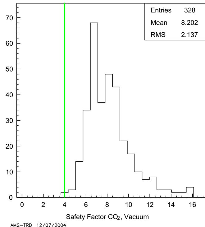
Fig. 6. AMS-02 TRD CO<sub>2</sub> gas tightness (safety factors) of the 328 flight straw modules.
