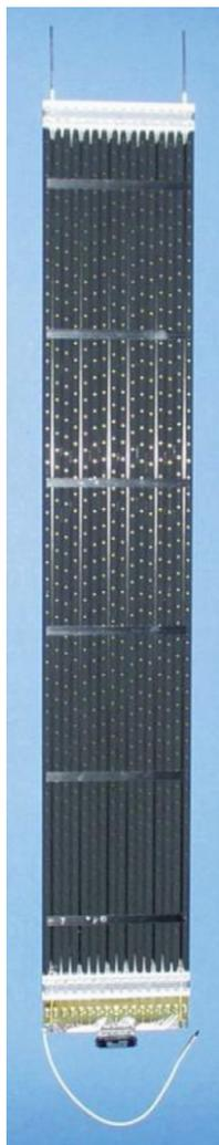
Fig. 1. AMS-02 TRD module with 16 straw tubes.
