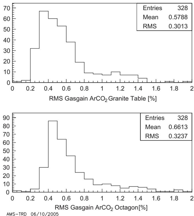
Fig. 5. AMS-02 TRD gas gain homogeneity of the 328 flight straw modules using Ar/CO<sub>2</sub> (80/20) at the nominal gas gain of 3000 before and after integration into the octagon support structure.
