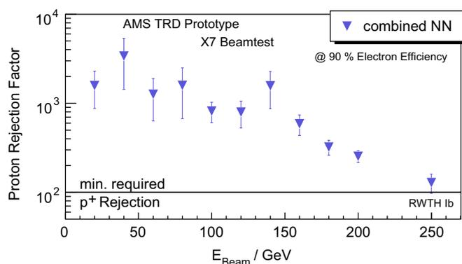
Fig. 8. AMS-02 TRD proton rejection.
