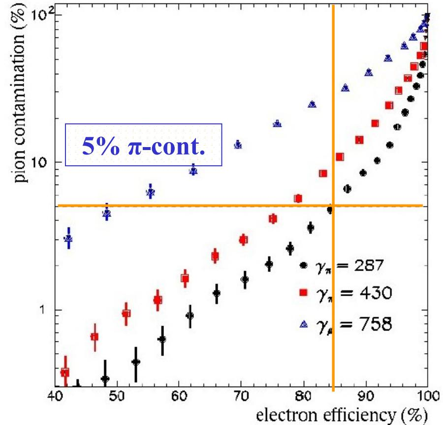
Rejection factor of 20 for non-radiating particles @ ~90 % e<sup>-</sup> efficiency
