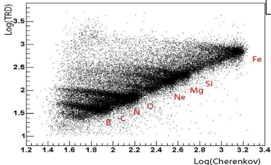
**Figure 3:** Measurements of the energy deposited in the TRD tubes versus the normalized Cherenkov light signal during the flight (~1 day).
