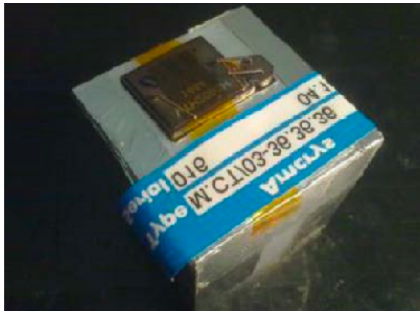
LYSO crystal with large and small area photodiodes glued to one face of the cube.
