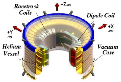
Figure 2.9: The superconducting magnet [27].
