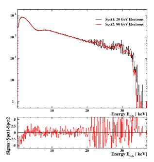
Figure 5.11: Comparison of 20 and 80 GeV electron spectra. Additionally plotted, is the difference of the two spectra's bin entries, normalised by the squared sum of the statistical errors.
