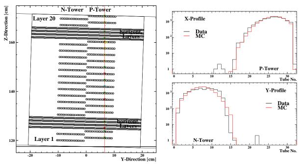
Figure 6.3: a) The prototype as defined for the MC simulations. Additionally plotted is the trajectory of a Proton that passed through the detector. The direction of the beam is from bottom to top; b) Comparison of the X- and Y-beam profiles of MC and data, plotted against the tube number hit in layer 1.
