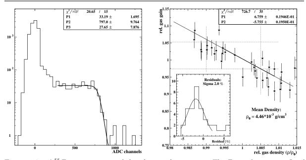
Figure 5.7: a)  ${}^{55}Fe$  spectrum recorded with a random trigger. The Fermi function is fitted to the upper edge to determine the photo-peak position [60]; b) Average gas gain value, derived from  ${}^{55}Fe$  spectra, as a function of gas density. A straight line fit is performed.
