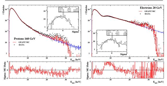
Figure 6.5: Comparison of Data and MC single tube energy spectra for a) 160 GeV protons and b) 20 GeV electrons. In both cases, the spectra without the implemented ADC cut-off, are plotted additionally.
