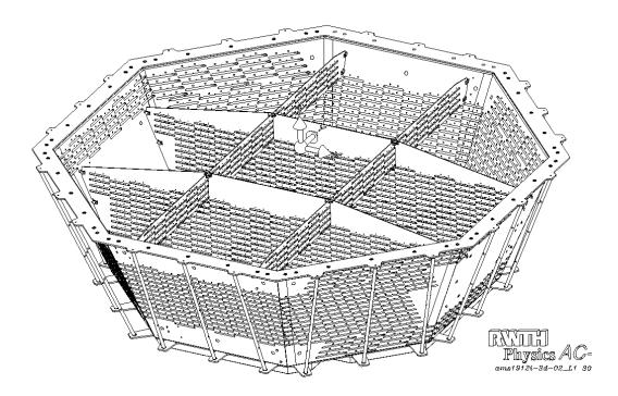
Figure 3.17: 3D view of the TRD octagon support structure [46, 49].
