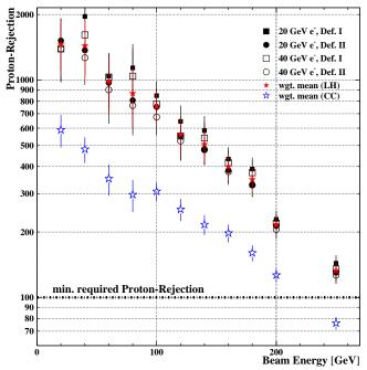
Figure 5.18: Proton rejection as a function of beam energy. Exponential declension down to a rejection (def.I) of  $(143 \pm 13)$  at 250 GeV proton energy. Additionally plotted is the average Cluster Counting distribution.
