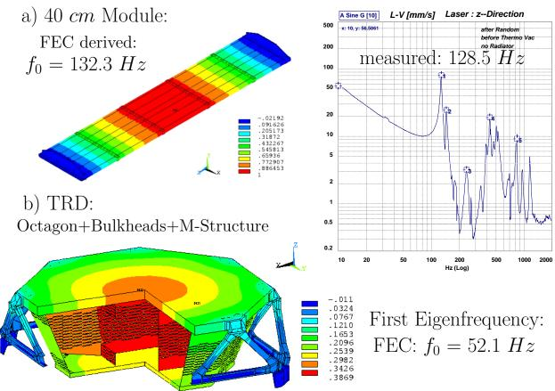
Figure 3.18: a) Z-displacement, derived from finite element calculations, for a 40 cm straw module and comparison of the calculated and measured first eigenfrequencies; b) Z-Displacement and eigenfrequency calculation for the TRD support structure (Octagon, Bulkheads and M-structure).
