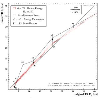
Figure 6.9: a) Comparison of detected TR photon energies before and after the tuning. Additionally plotted is the principal of the tuning along a set of 4 straight lines, defined by 6 parameters and 3 scale factors.
