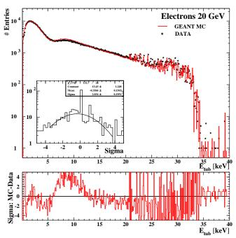
Figure 6.8: Comparison of Data and MC electron spectra. The MC spectrum has the dE/dx adjustment applied. The mean number of generated TR photons is reduced to 99 %.
