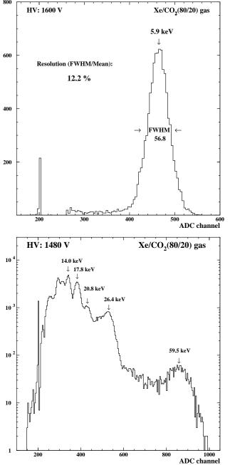
Figure 4.4: a)  ${}_{26}^{55}Fe$  spectrum; b)  ${}_{95}^{241}Am$  spectrum detected in  $Xe/CO_2$  gas, at NTP and the indicated annode voltages.
