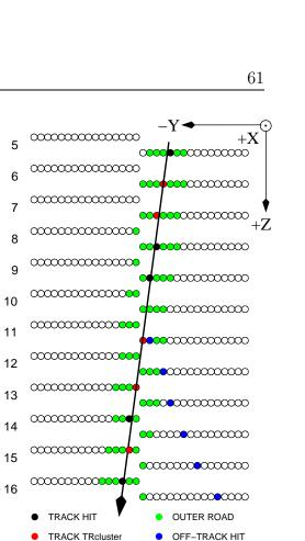
Figure 5.2: Principle of the track reconstruction in the vertical layers.
