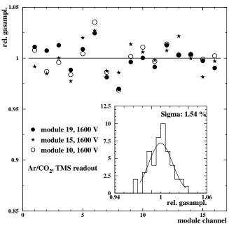
Figure 4.5: Homogeneity distributions accumulated from 3 prototype modules.
