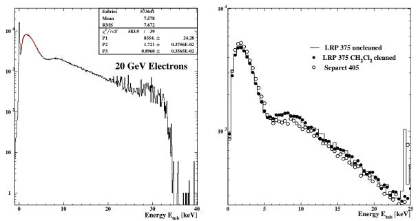
Figure 5.10: a) 20 GeV electron spectrum, containing the hits on the track of all selected single track events, recorded during the X7 beamtest; b) comparison of  $e^-$  spectra from, at each case, 3 successive layers with the same radiator material in front.
