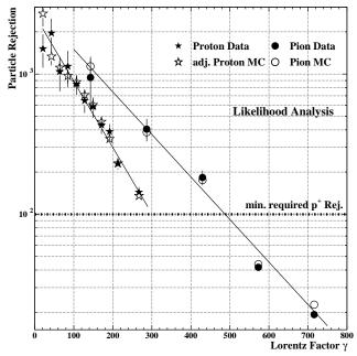
Figure 7.1: MC and Data particle rejection factors versus Lorentz factor  $\gamma$ .
