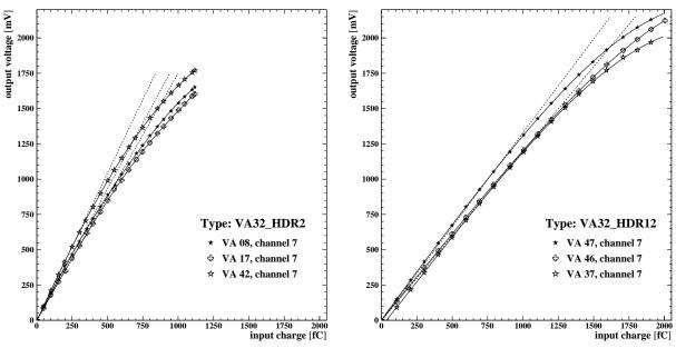
Figure 4.12: a) Gain linearity of the VA32\_HDR2 chips, used for the prototype; b) Gain linearity of the VA32\_HDR12 chips, proposed for the final TRD.
