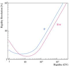
Figure 2.8: Momentum resolution of the Silicon-Tracker [24].
