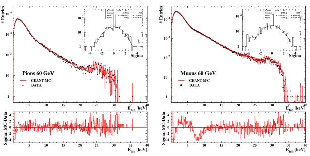
Figure 6.11: Comparison of the Data and final MC single tube energy spectra for a) 60 GeV Pions and b) 60 GeV Muons.
