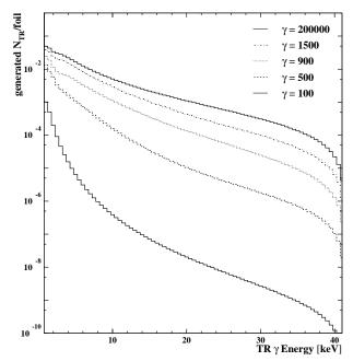
Figure 6.2: Simulation of TR generation. Integral number of generated TR photons, in a stack of foils, as a function of TR photon energy threshold, displayed for 5 different  $\gamma$  factors.
