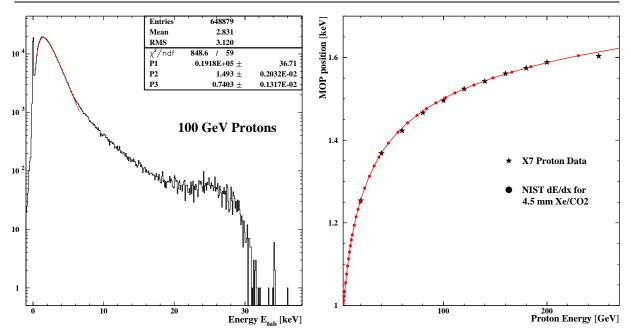
Figure 5.9: a) 100 GeV proton spectrum, containing the hits on the track of all selected single track events, measured during the X7 beamtest; b) Spectra's MOP position as a function of particle energy, compared to a calculated distribution from NIST.
