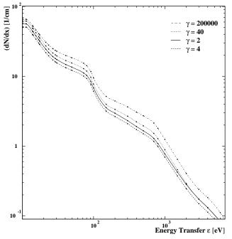
Figure 6.1: Ionisation energy loss simulation. Energy transfer distributions in  $Xe/CO_2$  gas for 4 different  $\gamma$  factors and stand. cond. (STP).
