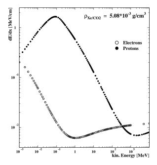
Figure 3.4: Calculated energy loss of electrons and protons in  $Xe/CO_2$ , at standard conditions (NTP), as a function of their kinetic energy according to Bethe-Bloch [37].
