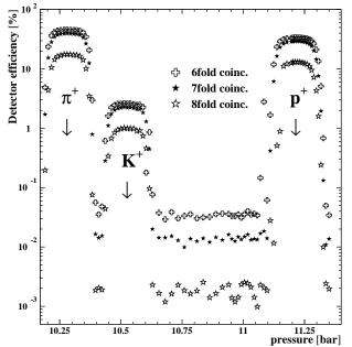
Figure 4.15: CEDAR efficiency as a function of gas pressure. The 6fold, 7fold and 8fold coincidence distributions are plotted for 120 GeV  $p^+$  energy, and an iris opening of 1 mm.
