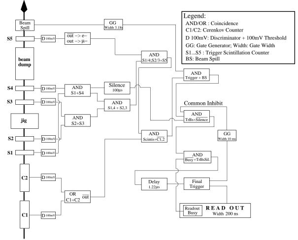
Figure 4.13: General beamtest set-up and trigger logic, as used for the X7-beamtest.
