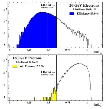
Figure 5.16: Likelihood distributions, on logarithmic scale, for the 20 GeV electron and the 160 GeV proton samples. The likelihood for events to be "electron-like" is plotted.
