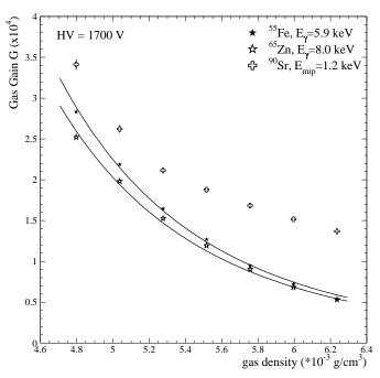
Figure 4.7: Gas gain as a function of gas density.
