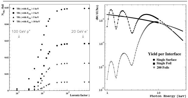
Figure 3.3: a) The increasing probability to generate a TR photon, from a single foil, up to the saturation at high  $\gamma$  factors; b) Calculated transition radiation yield normalised to one surface, from one surface, one foil and a stack of 200 foils, with 20 µm thickness and a 200 µm spacing. Transitions: air  $\Leftrightarrow$  Mylar and  $\gamma = 8000$  [34].
