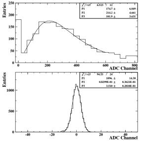
Figure 5.3: a) Landau fit to a single tube spectrum; b) Pedestal position after correction.
