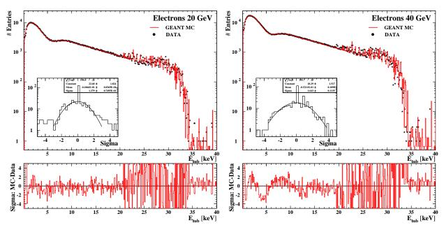
Figure 6.10: Comparison of the Data and final MC single tube energy spectra for a) 20 GeV and b) 40 GeV electrons.
