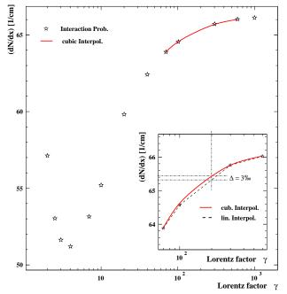
Figure 6.6: Ionisation energy loss simulation. number of interactions per cm versus  $\gamma$  factor, Embedded: The comparison between linear and cubic interpolation.
