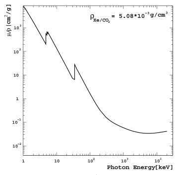
Figure 3.6: Absorption coefficient in a  $Xe/CO_2$  gas as a function of  $\gamma$  energy [39].
