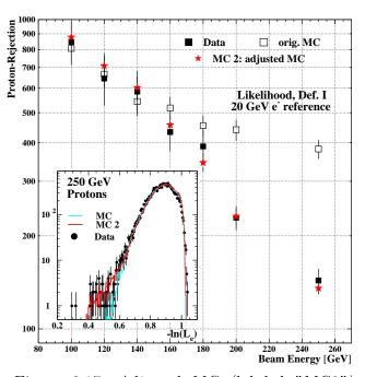
Figure 6.17: Adjusted MC (labeled "MC2") rejection factors as a function of beam energy in comparison to the data distribution. Embedded: Comparison of the Likelihood distributions from 250 GeV proton data and MC2.
