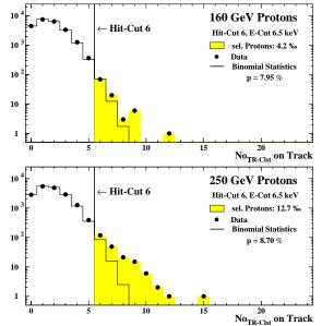
Figure 5.14: Hit-Cut distributions in comparison to the appropriate binomial distributions, with parameters n=20 and p, the fraction of entries, above the applied Ecut, here 6.5 keV, of the total energy spectrum.
