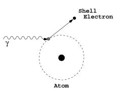
Figure 3.5: Schematic illustration of the photoelectric effect.
