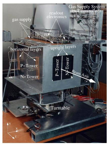
Figure 4.10: Photo of the 20-layer TRD prototype.
