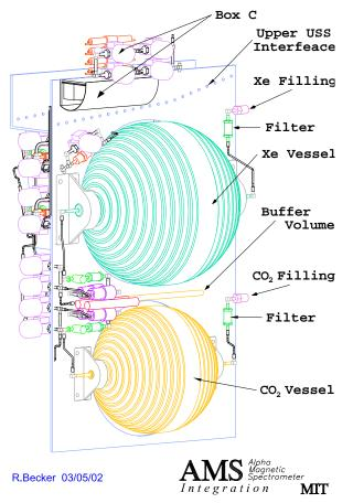
Figure 3.16: TRD gas supply system [22].
