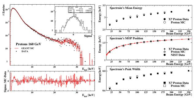
Figure 6.7: Comparison of Data and MC proton spectra. Left) Data and MC single tube energy spectra for 160 GeV protons; Right) Comparison of the spectra's mean energies, MOP positions and widths for all proton energies.
