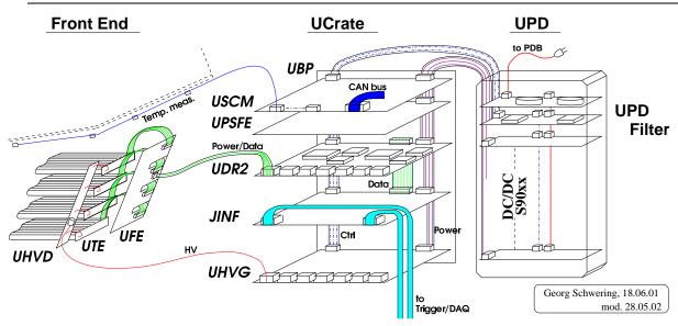
Figure 3.14: TRD electronics design.
