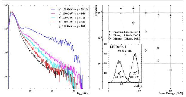
Figure 5.21: a) Energy spectra recorded with particles at various different Lorentz factors; b) Pion & muon rejection factor as a function of beam energy. Exponential declension down to  $(19.2 \pm 0.7)[(5.7 \pm 0.1)]$  at 100 GeV pion [muon] energy. For comparison the average likelihood distribution from the proton analysis is additionally plotted. Embedded; Likelihood distributions for 40 GeV pions compared to that of 20 GeV electrons.
