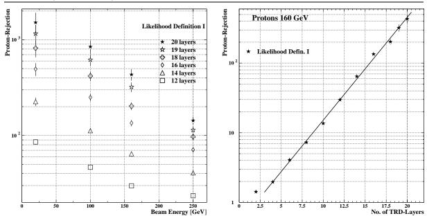
Figure 5.20: Proton rejection as a function of active layer number. Rejections are calculated from Likelihood definition I. a) Layer variation from 20 down to 12 active layers for 4 different proton energies; b) Layer variation from 20 down to 2 active layers, performed for 160 GeV proton energy.
