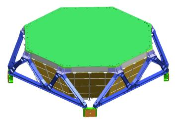
Figure 2.14: The transition radiation detector with the M-support structure [22].
