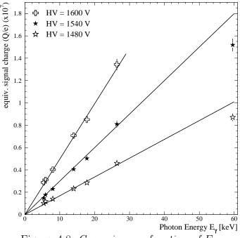
Figure 4.8: Gas gain as a function of  $E_{\gamma}$ .
