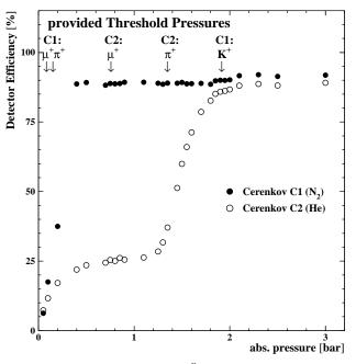
Figure 4.14: Threshold Čerenkov detector efficiencies as functions of gas pressure, for the two counters, filled with He or  $N_2$  gas, respectively, obtained for  $E_{beam} = +15 \text{ GeV}$ .
