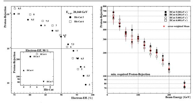
Figure 5.13: a)  $p^+$ -rejection as a function of  $e^-$ -efficiency. Attached numbers indicate the applied Ecut [keV]. Embedded; Dependence of the  $p^+$ -rejection on the Hit – Cut, at 90 % efficiency; b) Proton rejection as a function of beam energy. Exponential declension down to an average rejection of (76 ± 5) at 250 GeV proton energy.
