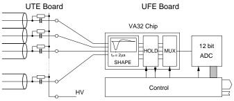
Figure 3.13: The front end electronics scheme.
