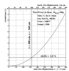
Figure 3.9: The effect of mechanical wire displacement on the gas amplification [41].
