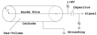
Figure 3.8: Schematic illustration of a proportional chamber [40].
