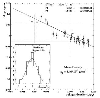
Figure 5.6: The relative change of the average gas gain factor, derived from MOP position of muon spectra, as a function of rel. gas density. A straight line is fitted to the distribution.
