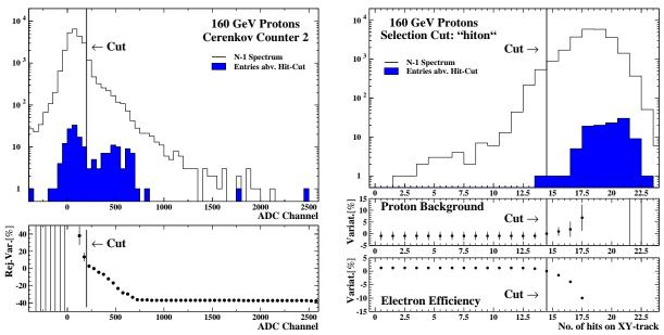
Figure 5.15: "n-1" distribution and variation of selected proton number for a) the second Čerenkov counter; b) the "hiton" selection cut. In this second case, the electron efficiency variation is additionally plotted.
