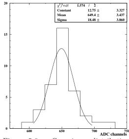
Figure 5.8: Gaussian distribution of energy calibration factors, derived from  ${}^{55}Fe$  measurements, taken throughout the X7 beamtest.
