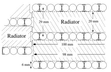
Figure 4.9: Zoom into the layer structure.
