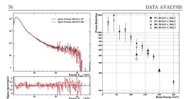
Figure 5.19: a) Comparison of the 160 GeV proton spectra recorded during the X7 and H6 beamtests; b) Proton rejection for the H6 beamtest data, derived from definition I, as a function of beam energy. Additionally plotted, is the equivalent proton rejection distribution from the X7 beamtest.
