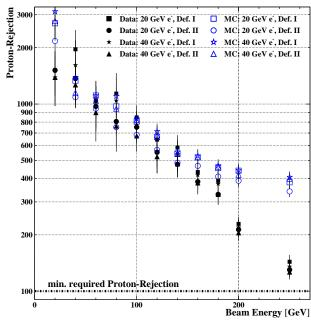
Figure 6.15: *MC* and data proton rejections, derived from definition I likelihood, as functions of beam energy.
