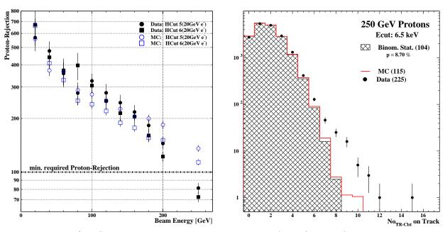
Figure 6.13: a) MC and data proton rejections, derived from Cluster Counting method, as functions of beam energy; b) Comparison of the MC and data proton Hcut distributions. Additionally plotted is the related distribution, derived from binomial statistics. The numbers, given in the brackets, indicate the entries above Hcut 6.
