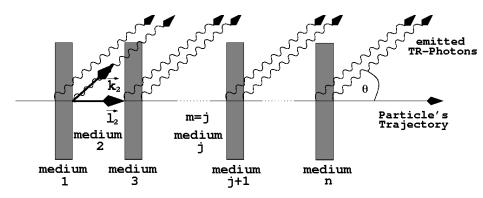
Figure 3.2: A charged particle traverses a stack of foils (dark shaded media), surrounded by air. The foil thickness is chosen such, that TR-photons emitted from the two foil boundaries constructively interfere.
