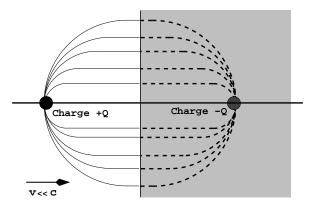
Figure 3.1: Electric charge in front of a perfectly conducting surface forms an electric dipole. Continuous and dashed lines represent the electric field lines.
