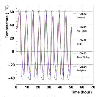
Figure 3.20: The 8 thermo-cycles of a thermo-vacuum test [51].
