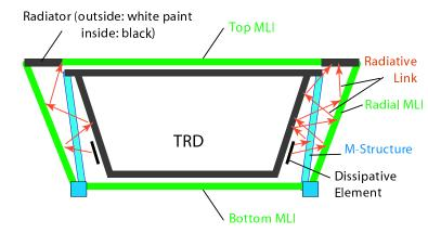
Figure 3.19: Thermal model of the TRD subsystem, wrapped in an Multi Layer Insulation.
