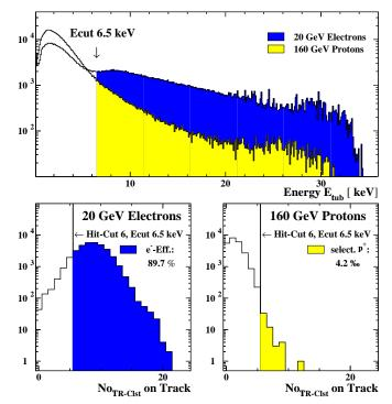
Figure 5.12: The Cluster Counting method. a) Energy-cut(Ecut) definition; b,c) The Hit - Cut is chosen such that the electron efficiency is 90 %.
