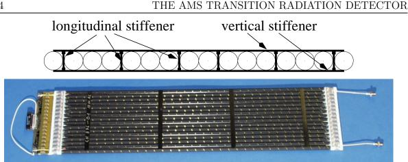
Figure 3.12: a) Cross section and b) photo of a straw module.
