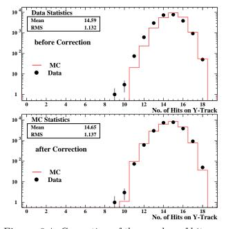
Figure 6.4: Correction of the number of hits on the Y-track. In the lower distribution the average number of hits in the Y-layers is randomly reduced in number down to 98%, compared to the original GEANT simulation.
