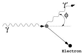
Figure 3.7: Schematic illustration of the Compton effect.
