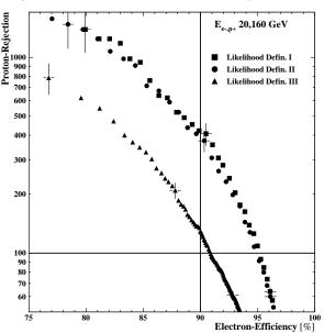
Figure 5.17: Proton rejections, derived from the three different likelihood definitions, as functions of electron efficiency. Error bars are only exemplary plotted to keep the distributions comparable.
