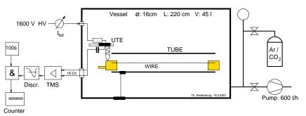
Figure 4.2: Schematic illustration of the Preview Test.
