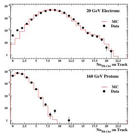
Figure 6.12: Comparison of MC and Data Hcut distributions for 20 GeV electrons and 160 GeV protons.
