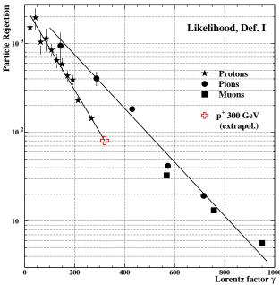
Figure 5.22: Particle rejections as a functions of the Lorentz factor,  $\gamma$ . Distributions show the expected exponential dependence on  $\gamma$ , where, on the logarithmic scale, the Proton distribution seems to have a significantly steeper slope compared to those from Pions and Muons.
