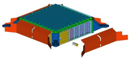
Figure 2.13: The electromagnetic calorimeter [22].
