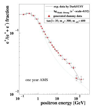
Figure 2.6: Positron fraction as expected after one year of AMS on the ISS, assuming a Neutralino of 240 GeV mass and a boost factor  $\sim 10^4$  [5].
