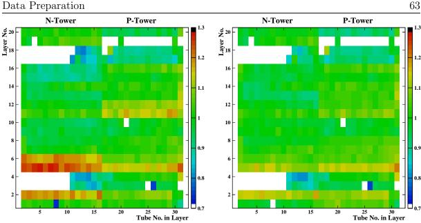
Figure 5.4: a) Inter-Calibration table from muon runs; b) VA gains corrected.
