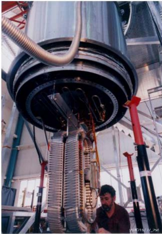
Figure 2.8: Testing the coils to flight loads.
