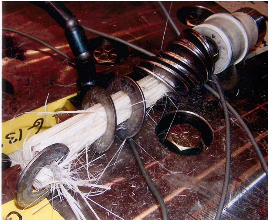
Figure 2.11: .Testing of strap to failure to understand the critical failure mode. Assembly failure caused by failure of the glass fiber “bod”, other damage observed caused by impact loading as strap failed, not by static loading.
