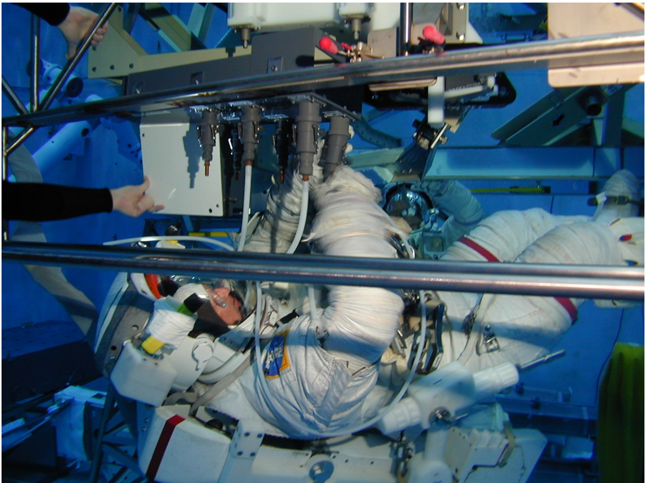
Figure 2.159: Practicing contingency EVA swap of AMS data cables at NBL.
