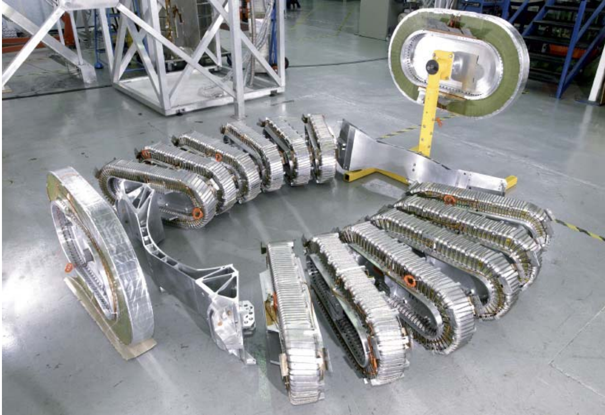
Figure 2.9: Arrangement of the completed 2 dipole coils, 12 flux return coils and structural members in roughly the positions they will have in the flight magnet.
