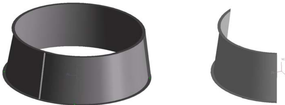
Figure 2.115: The conical reflector of the Cerenkov detector (3 sectors layout).
