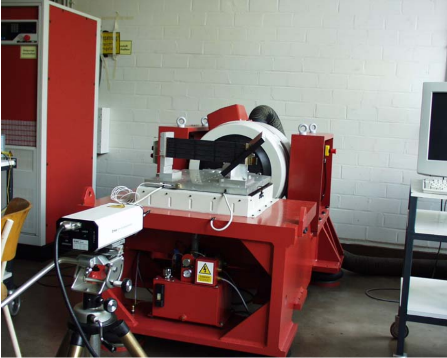
Figure 2.29: Vibration test stand loaded with a TRD straw module at RWTH-Aachen.
