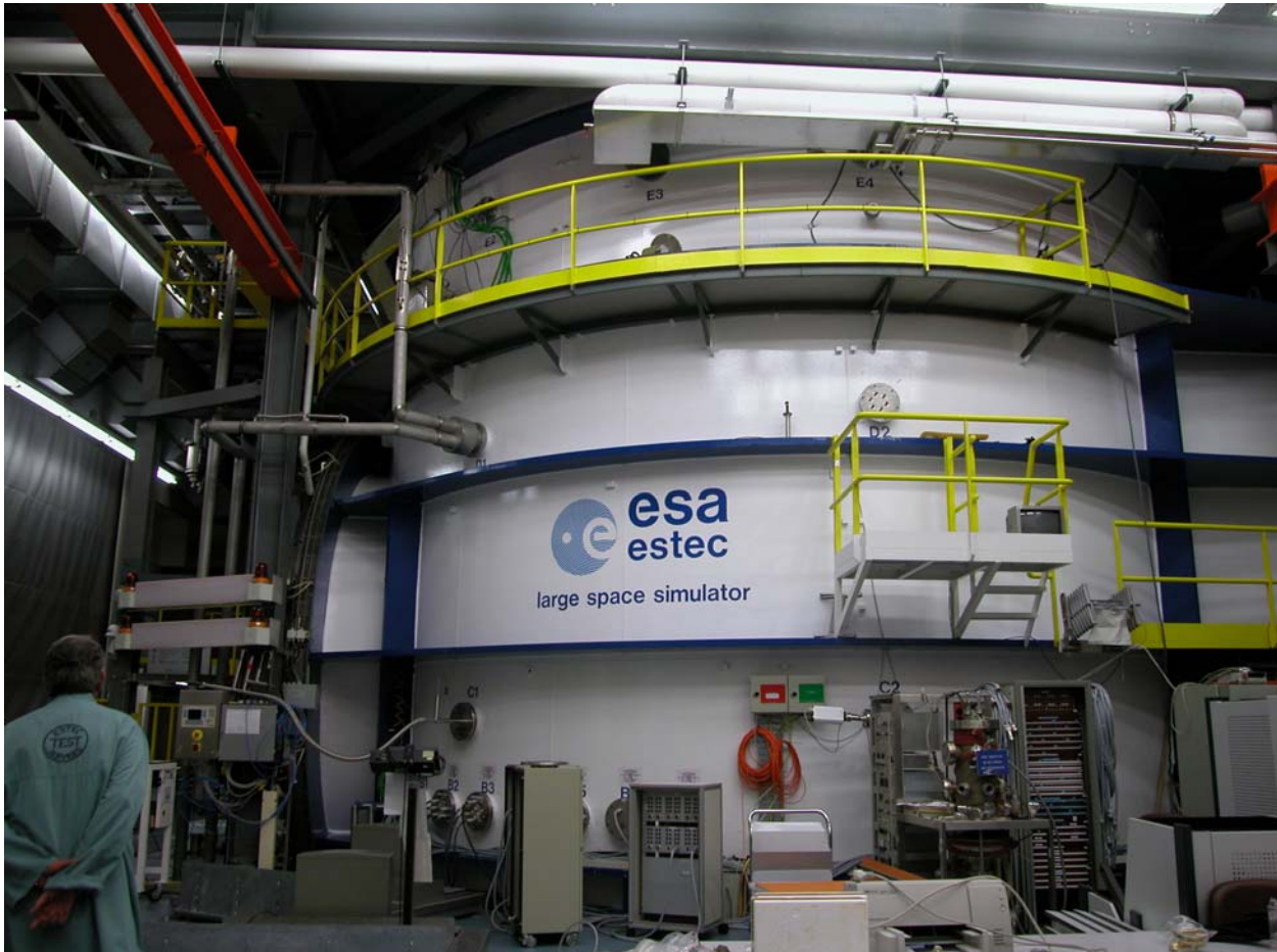
Figure 2.200: The Large Space Simulator (LSS) at ESTEC, site of the AMS thermal vacuum test.
