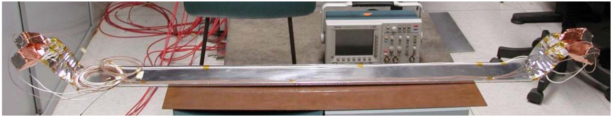
Figure 2.92: Design of a TOF paddle and photograph of an assembled paddle after thermal vacuum and electrostatic discharge tests.
