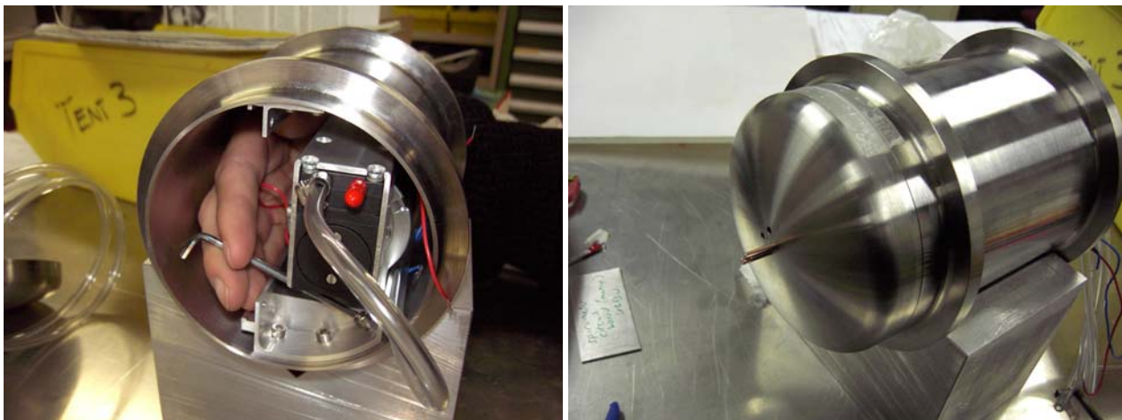
Figure 2.54: Left - Engineering model of Box C vessel with pump visible at in the opening. Right - Vessel with end cap in place and gas feedthrough.
