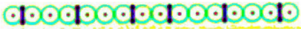
Figure 2.31: TRD Module Computer Tomography. The straw walls and the central wires are clearly visible.
