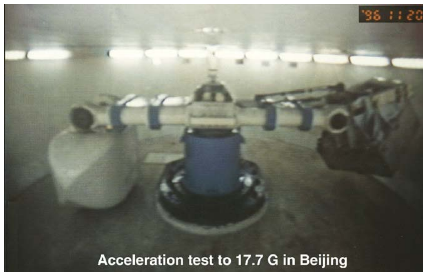
Figure 1.4: AMS-01 magnet undergoing centrifuge (static load) testing at the Laboratory for Centrifugal Modeling in Beijing, China.
